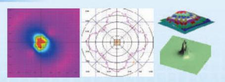
The temperature distribution on a finished PCB may be analyzed graphically with the help of Thermal Analyzers. The result of the analysis is displayed using isotherms or color mapping schemes.
