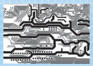
copper removal is also implemented. Final artworks are prepared for photo plotting. EDWinXP supports both standard (RS-274D) and extended (RS-274X) Gerber ASCII formats. The powerful Gerber ASCII file viewer is integral part of this module, enabling verification of artwork prior to plotting and fabrication.
